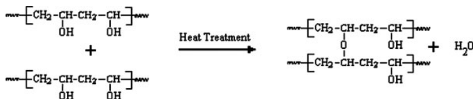
Scheme 2 Proposed reaction mechanism for crosslinking PVA membranes.
